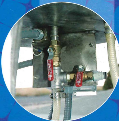
VALVES TO BYPASS SPRAY BALL TO CLEAN IN PLACE EQUIPMENT.
