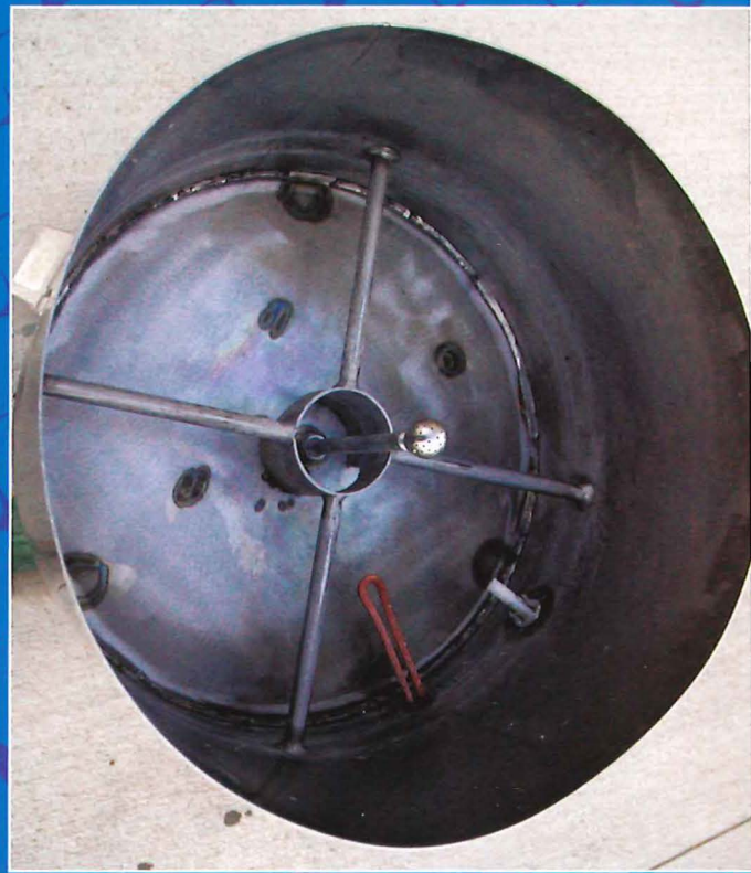
HEATER ELEMENT COPPER COLOR, WHITE SWITCH IS A LEVEL SWITCH, NEVER WIRED IN PLACE, DRAIN TOP LEFT, SPRAY BALL.
